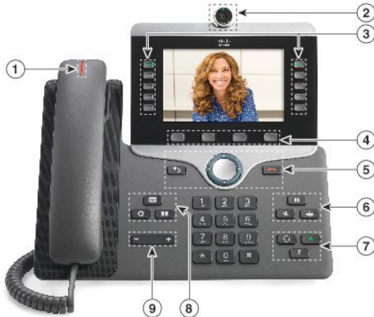
Figure 2: Cisco IP Phone 8800 Buttons and Hardware
