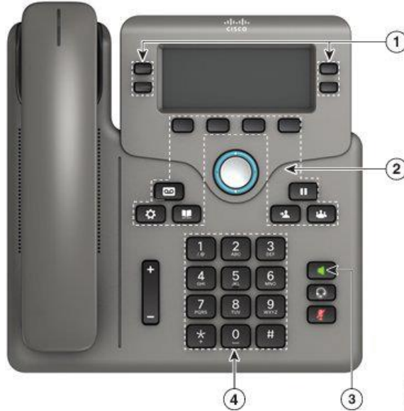
Figure 6: Mobility-Impaired Accessibility Features
